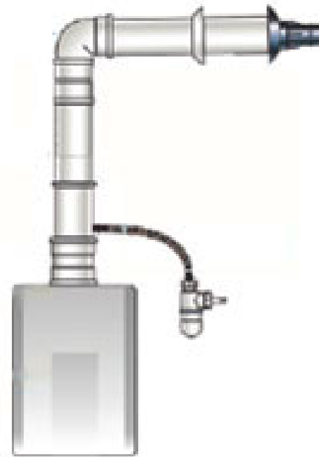
Horizontal venting with condensate trap
