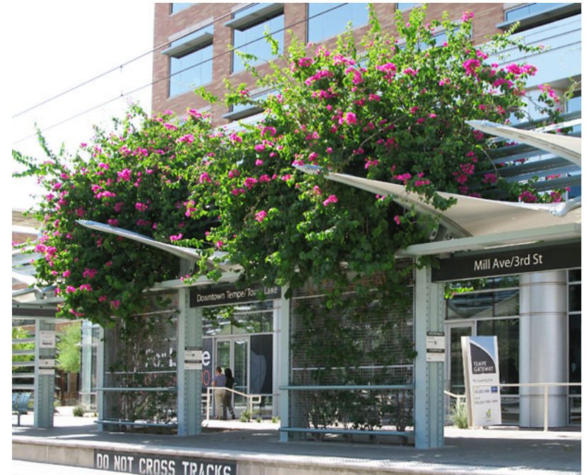
The facade plants are pruned at the pedestrian level to create a shade canopy above, Valley Metro Light Rail, Tempe, AZ.
