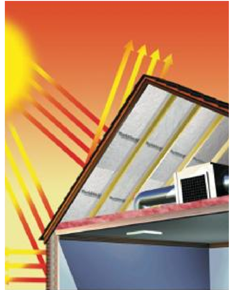
Summer radiant gain deflected with radiant barrier
