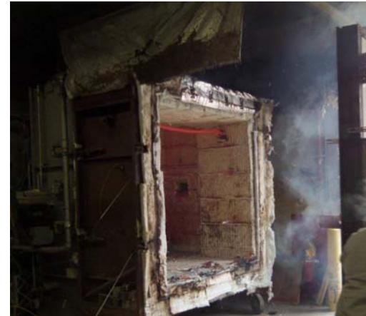
Frame is removed from the furnace.
