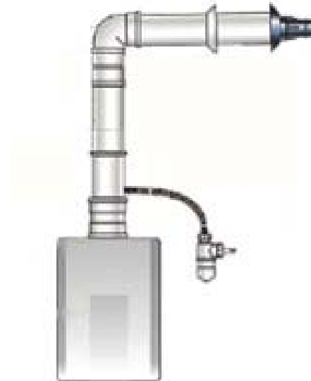
Horizontal venting with condensate trap
