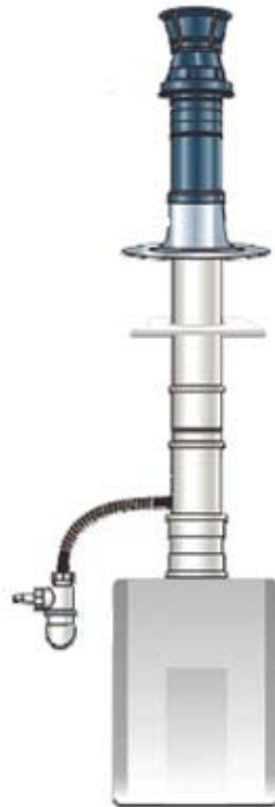
Vertical venting with condensate trap
