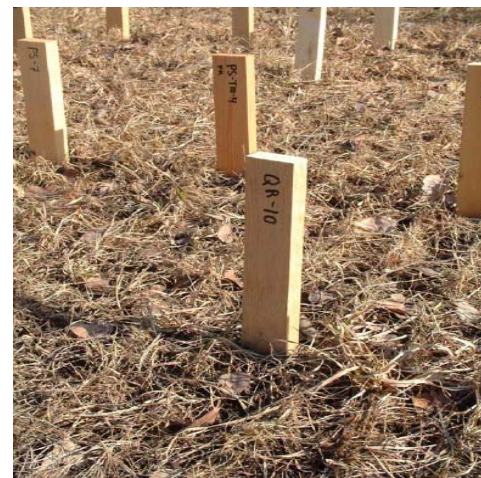
EN252 “Field test method for determining the relative protective effectiveness of a wood preservative in ground contact”
