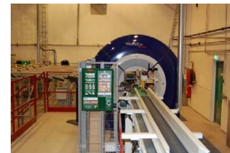
Quality control scanner
