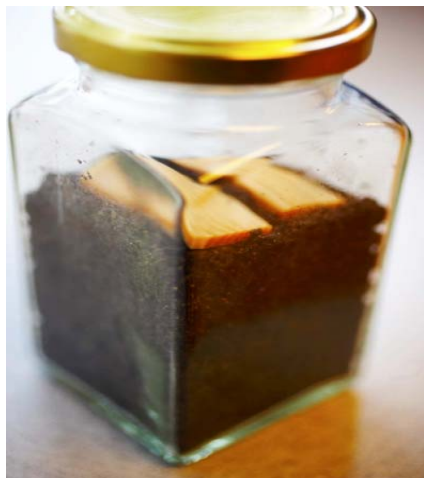
AWPA E10 “Standard Method of Testing Wood Preservatives by Laboratory Soil-Block Culture”
