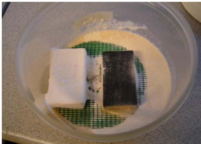
EN113 “Wood preservatives. Test method for determining the protective effectiveness against wood destroying basidiomycetes. Determination of the toxic values”
