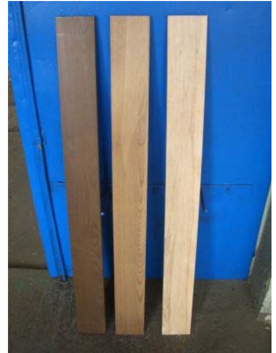
Thermally modified beech (sample on right is untreated)
