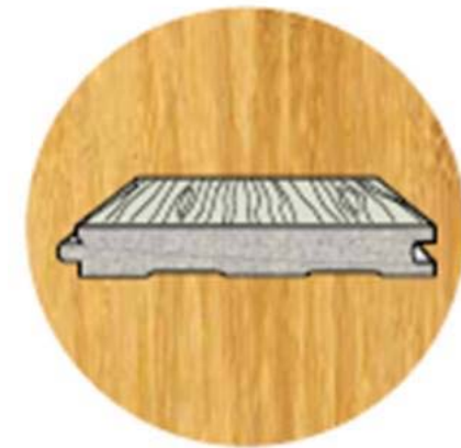
Cross-Section: Flooring Plank Made of Solid Strand Bamboo
