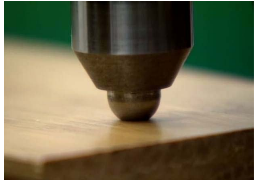
Janka Hardness Test Measures force needed to embed ball
