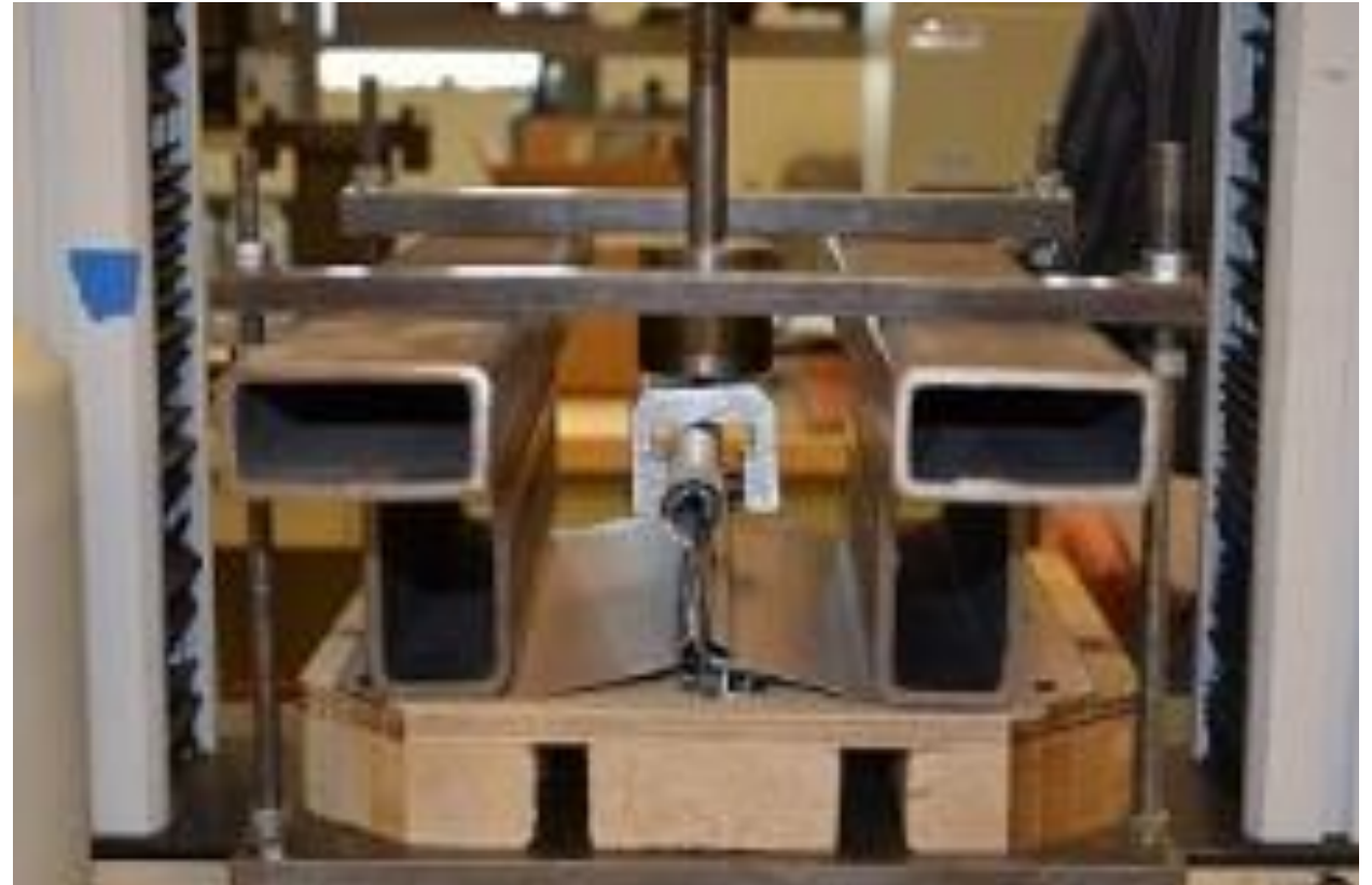
Pull-off test with a universal fit aluminum clamp using three stainless steel, cupped tip set screws on a Morin bulb seam. This clamp far exceeds the strength of the super strong panel joint.
